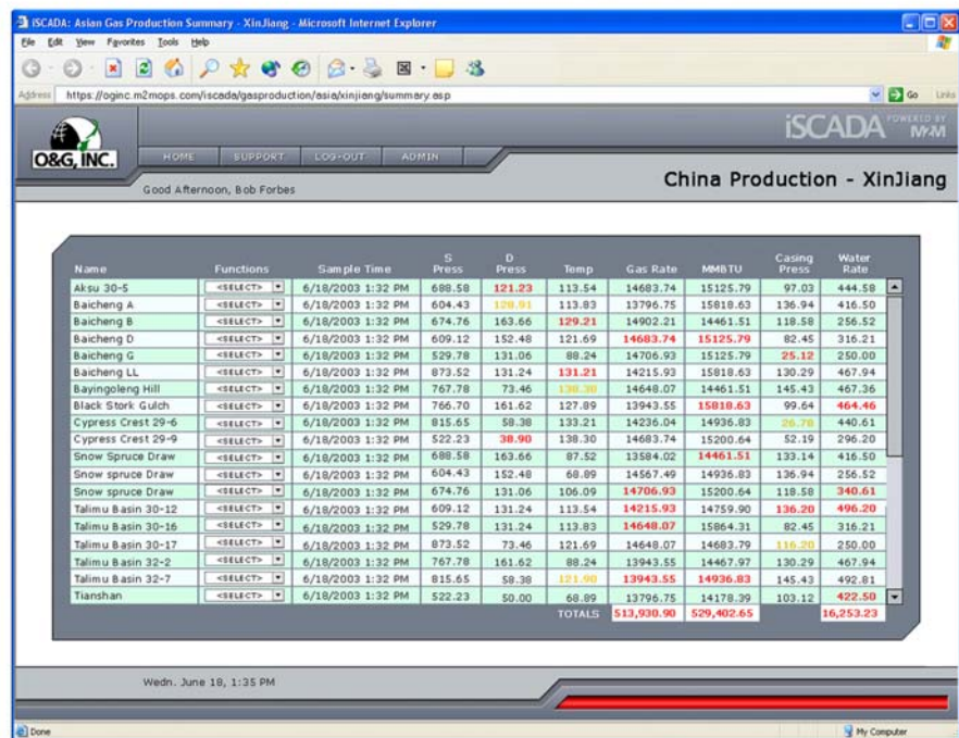
FIG. 2: Summary of gas production wells in XinJiang, China. M2M's iSCADA relays this information to owners and operators wherever they are located.
